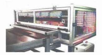
to size. The knife assembly is servo driven with linear guides for extra strength and support. Easy to use, the unit can be bolted right into an existing process. A color touch screen is used to set up the unit. PLC controls run the servo motor drive and the entire process. To interface the unit to the process, a loop sensor is used. When material is present, the unit will operate; if there is no material, it will wait.
